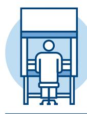
Per CDC guidelines, primary barriers such as biosafety cabinets should be used when procedures might cause splashing of droplets – including pipetting, shaking and opening containers of infectious materials (2).
